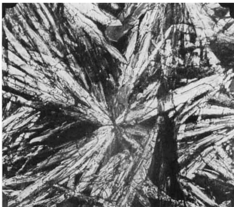
FIGURE 9 Solid I phase formed on heating the quenched sample. Magnification \times 300 .
