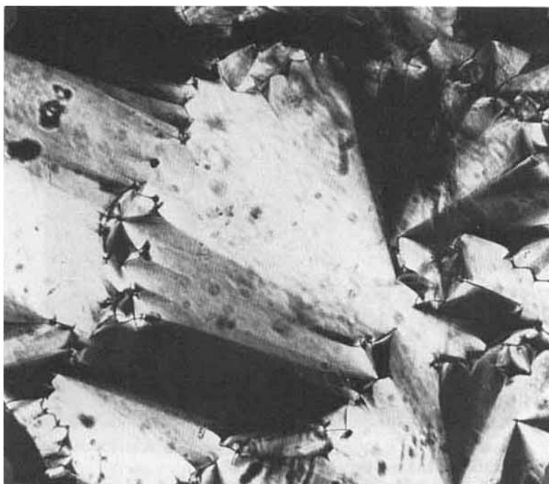
FIGURE 3 Smectic B phase in a cooled sample. Magnification \times 135 at 26^{\circ}\text{C} .
