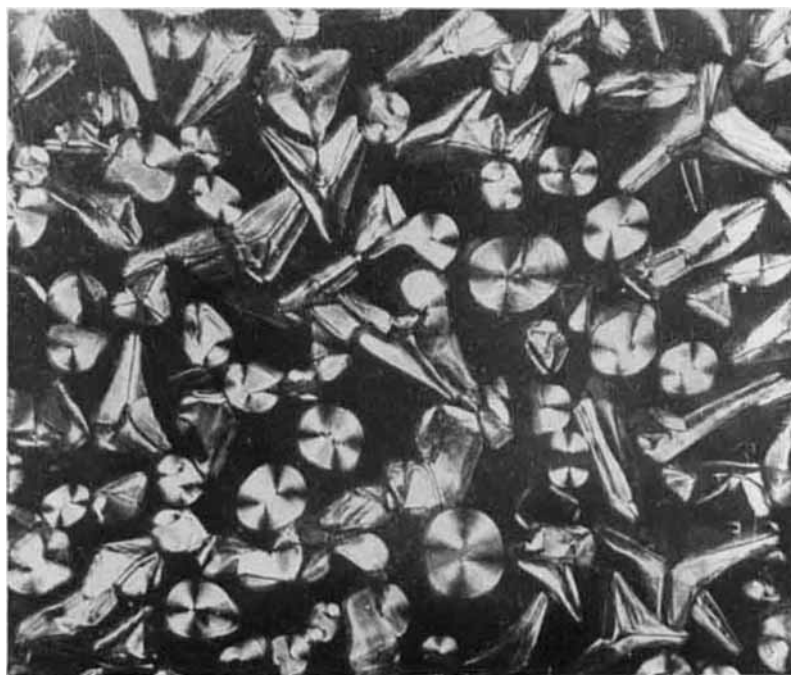
FIGURE 7 Spherulites formed on quenching the sample to 26^{\circ}\text{C} from its isotropic phase. Magnification \times 135 .
