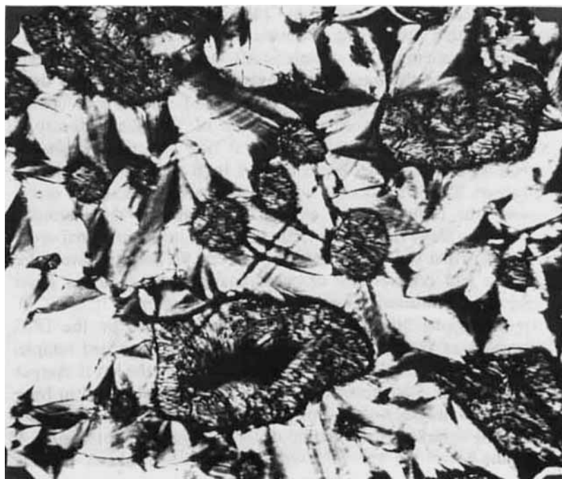
FIGURE 6 Smectic A-Cholesteric transition magnification \times 135 .
